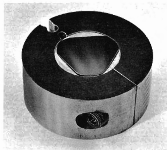
FIG. 1 Adjustable jig used in lapping and polishing of semiconductor plates.
