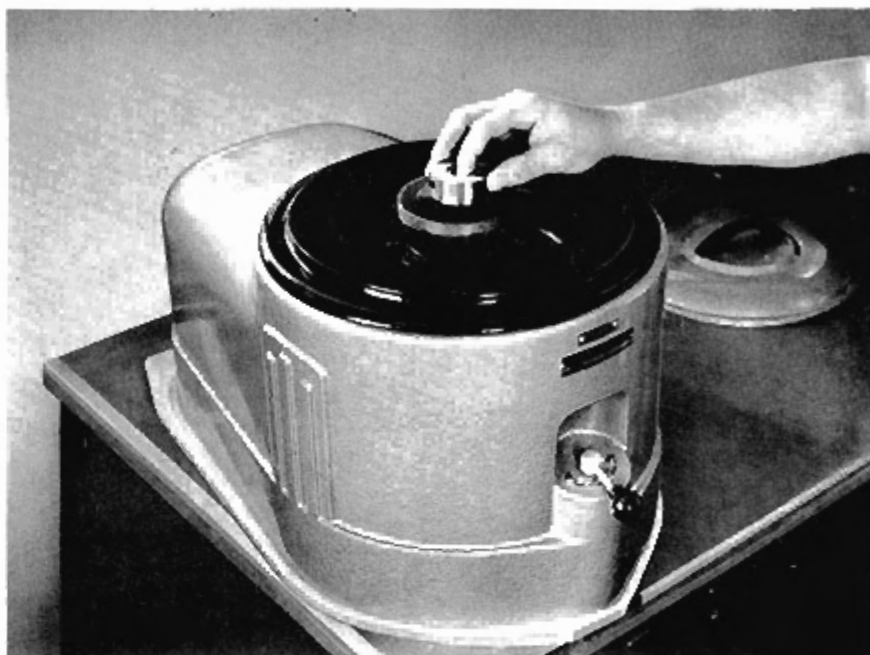
FIG. 3 Final polishing with \frac{1}{2}\mu diamond abrasive on rayon covered lap.
