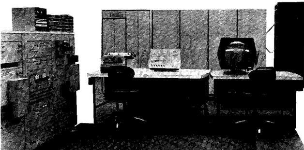
Some of the first PDP-1's had graphic display systems as peripherals. These were the first commercially available graphic terminals for computers. Although the last PDP-1 was built in 1969, nearly all 53 PDP-1's are still in use, most of them in universities. Some of the applications of this machine included message switching, instrument control, and special purpose timesharing.
