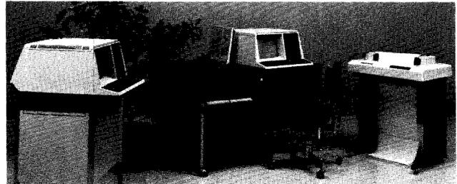
The Datasystem 322 is a floppy diskette based system with 32K bytes of memory packaged in the same desk as the DS310 and using a VT52 CRT. It can be configured with more memory, additional terminals, more mass storage, and a variety of printers.
