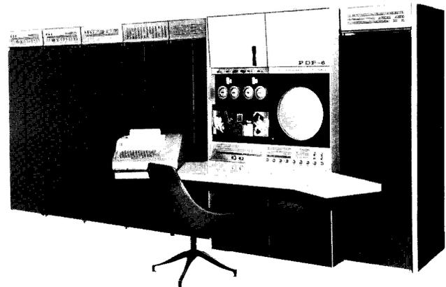
M.I.T., were previously available, but none had manufacturer support. Some new techniques, including larger system units, were used in the twenty-three PDP-6 systems installed.
